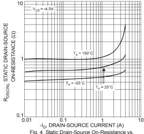
Fig. 4 Static Drain-Source On-Resistance vs.
