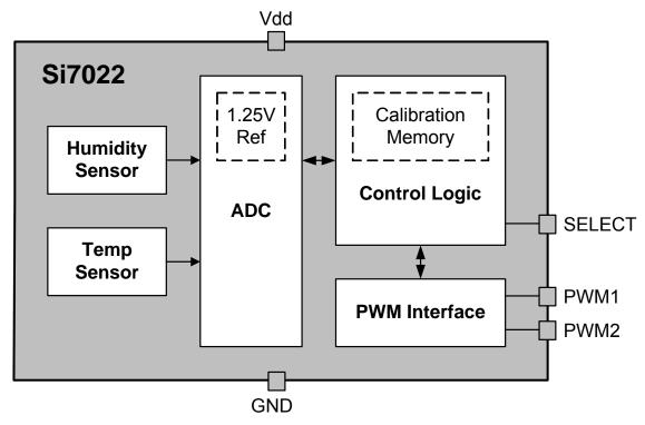
Figure 5. Si7022 Block Diagram
