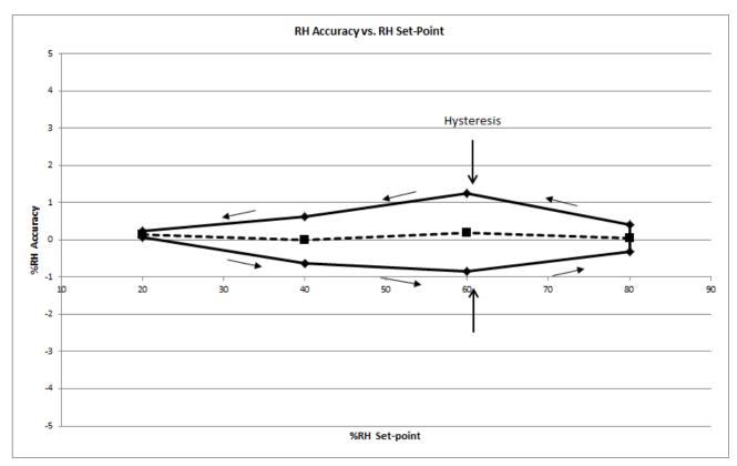
Figure 6. Measuring Sensor Accuracy Including Hysteresis
