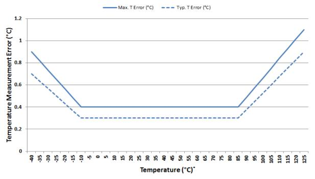
Figure 3. Temperature Accuracy
