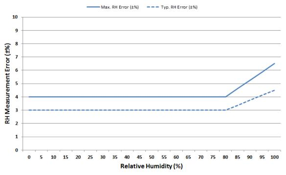
Figure 2. RH Accuracy at 30 °C
