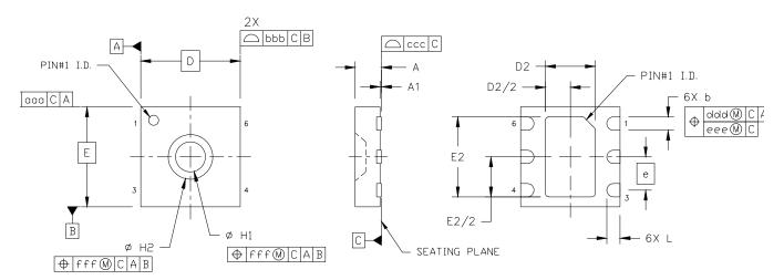
Figure 10. 3x3 6-pin DFN
