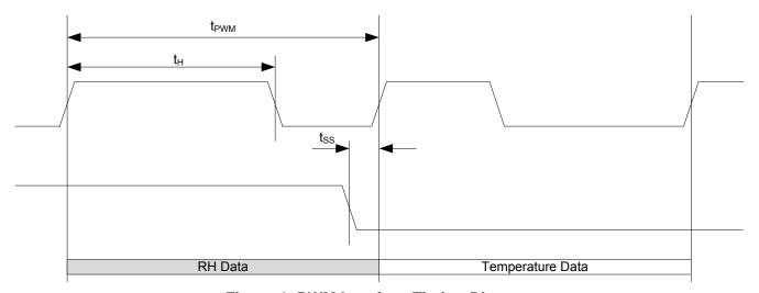
Figure 1. PWM Interface Timing Diagram
