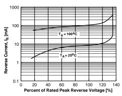
Figure 4. Reverse Current vs Reverse Voltage
