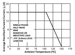
**Figure 1. Forward Current Derating Curve**
