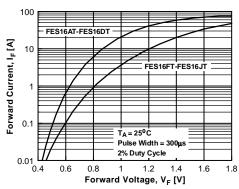
Figure 3. Forward Voltage Characteristics
