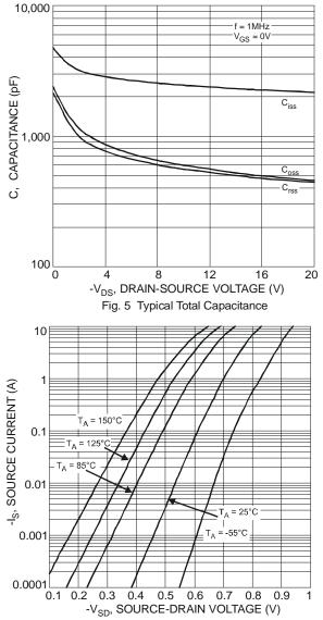
Fig. 7 Reverse Drain Current vs. Source-Drain Voltage
