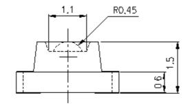
For reflow soldering (propose)
