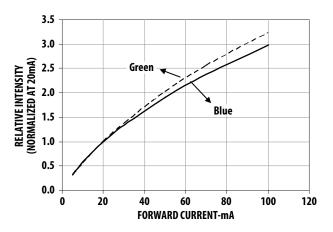
Figure 7. Relative Intensity vs Forward Current
