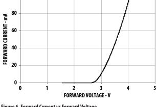
Figure 6. Forward Current vs Forward Voltage
