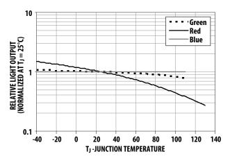
Figure 12. Relative Light Output vs Junction Temperature
