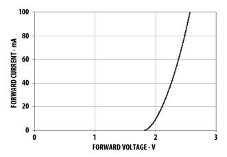
Figure 2. Forward Current vs Forward Voltage
