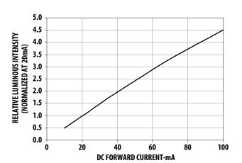
Figure 3. Relative Intensity vs Forward Current
