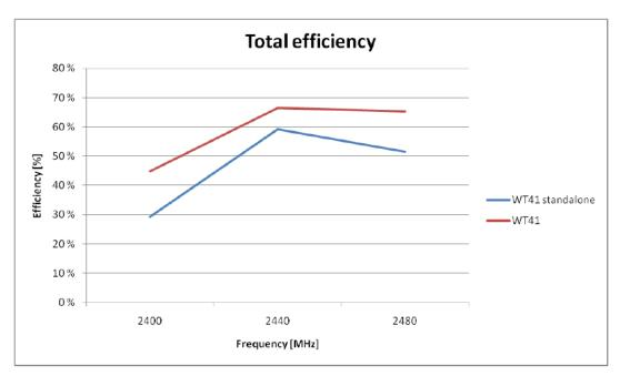
Table 14: Total efficiency of the chip antenna
