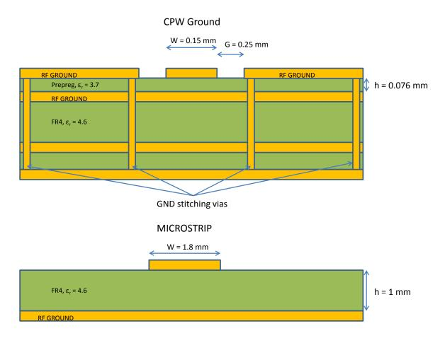
Figure 12: Example cross section of two different 50 ohm transmission line
