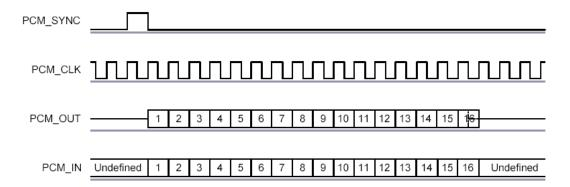
Figure 22: Short Frame Sync (Shown with 16-bit Sample)
