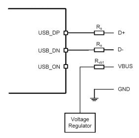
Figure 17: USB Connections for Bus-Powered Mode
