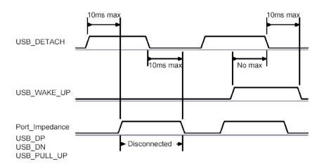
Figure 18: USB Detach and USB Wake Up Signals
