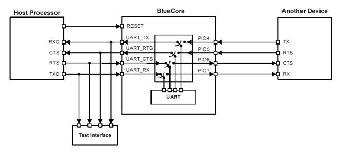
Figure 14: UART Bypass Architecture
