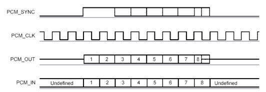
Figure 21: Long Frame Sync (Shown with 8-bit Companded Sample)
