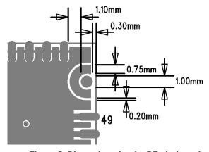
Figure 5: Dimensions for the RF pin (top view)
