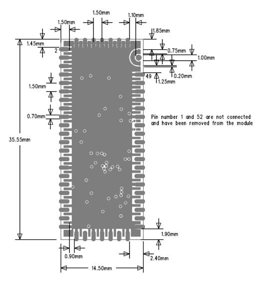
Figure 4: Physical dimensions (top view)
