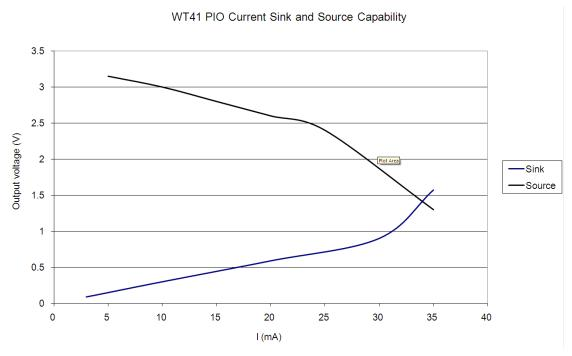
Figure 2: WT41 PIO Current Drive Capability
