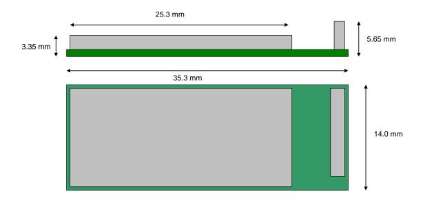
Figure 6: Dimensions of WT41
