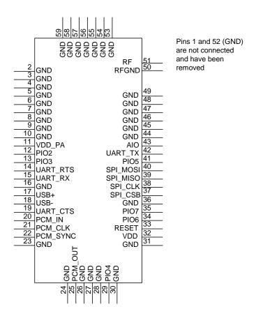
Figure 1: WT41 pin out
