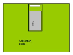
Figure 8: Recommended positions for WT41-A
