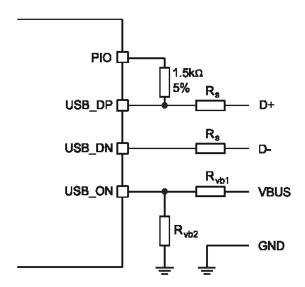
Figure 15: USB Connections for Self-Powered Mode
