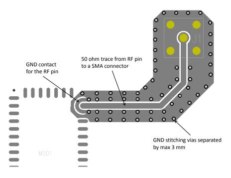
Figure 11: Example RF trace for WT41-N
