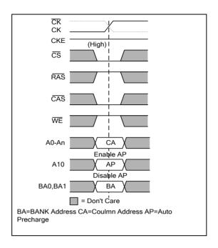
The basic Read timing parameters for DQs are shown in following figure; they apply to all Read operations.
