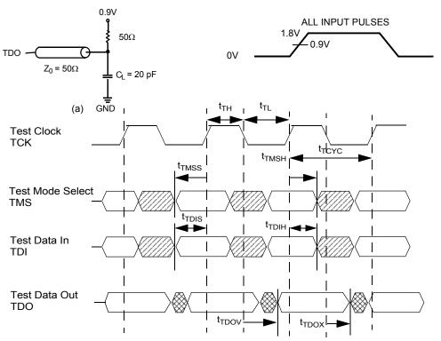
Figure 3. TAP Timing and Test Conditions
