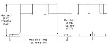
Note: Allow air circulation within the sealed type G8P by removing the ventilation nib from the cover after soldering and cleaning is complete.
