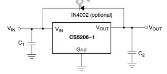
Figure 12. Protection Diode Scheme for Fixed Output Regulators
