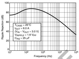
Figure 9. Ripple Rejection vs. Frequency (Adjustable Version)
