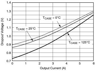
Figure 3. Dropout Voltage vs. Output Current
