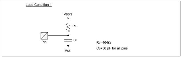
TABLE 4-9: CAPACITIVE LOADING REQUIREMENTS ON OUTPUT PINS
