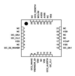
**Note:** The metal plane at the bottom of the device is not connected to any pins and is recommended to be connected to VSS externally.
