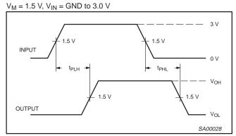
Waveform 1. Input (An) to Output (Yn) Propagation Delays
