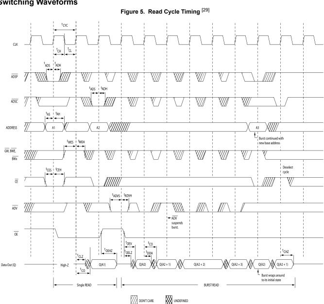
29. On this diagram, when  $\overline{CE}$  is LOW:  $\overline{CE}_1$  is LOW,  $\overline{CE}_2$  is HIGH and  $\overline{CE}_3$  is LOW. When  $\overline{CE}$  is HIGH:  $\overline{CE}_1$  is HIGH or  $\overline{CE}_2$  is LOW or  $\overline{CE}_3$  is HIGH.
