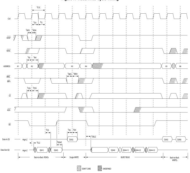
32. On this diagram, when  $\overline{CE}$  is LOW:  $\overline{CE}_1$  is LOW,  $\overline{CE}_2$  is HIGH and  $\overline{CE}_3$  is LOW. When  $\overline{CE}$  is HIGH:  $\overline{CE}_1$  is HIGH or  $\overline{CE}_2$  is LOW or  $\overline{CE}_3$  is HIGH. 33. The data bus (Q) remains in high Z following a WRITE cycle, unless a new read access is initiated by  $\overline{ADSP}$  or  $\overline{ADSC}$ .
