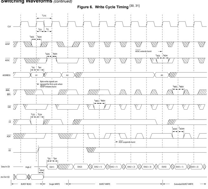
30. On this diagram, when  $\overline{CE}$  is LOW:  $\overline{CE}_1$  is LOW,  $\overline{CE}_2$  is HIGH and  $\overline{CE}_3$  is LOW. When  $\overline{CE}$  is HIGH:  $\overline{CE}_1$  is HIGH or  $\overline{CE}_2$  is LOW or  $\overline{CE}_3$  is HIGH. 31. Full width write can be initiated by either  $\overline{GW}$  LOW; or by  $\overline{GW}$  HIGH,  $\overline{BWE}$  LOW and  $\overline{BW}_X$  LOW.
