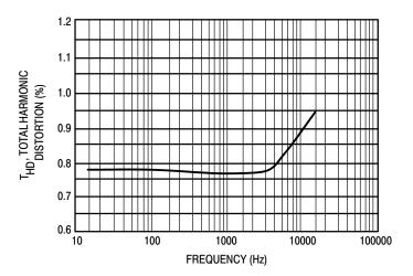
Figure 16. Typical Total Harmonic Distortion
