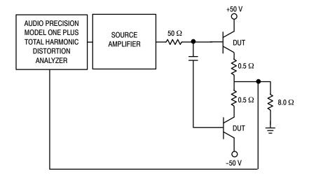
Figure 17. Total Harmonic Distortion Test Circuit
