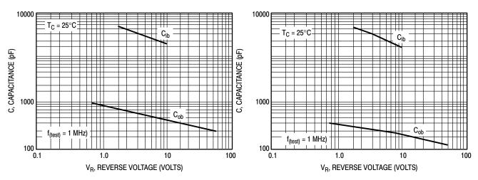
Figure 14. MJL21193 Typical Capacitance
