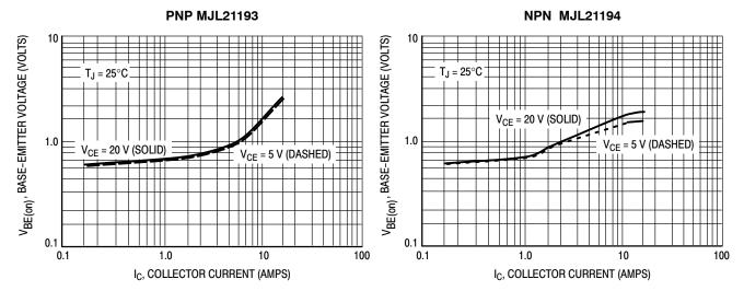
Figure 11. Typical Base-Emitter Voltage
