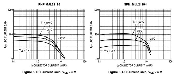
Figure 5. DC Current Gain, V<sub>CE</sub> = 5 V
