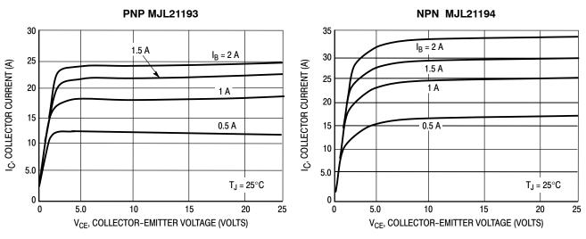
Figure 7. Typical Output Characteristics
