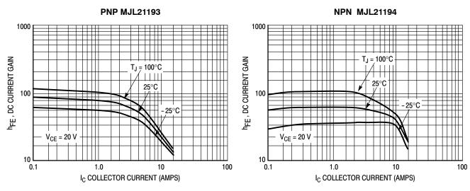
Figure 3. DC Current Gain, V<sub>CE</sub> = 20 V
