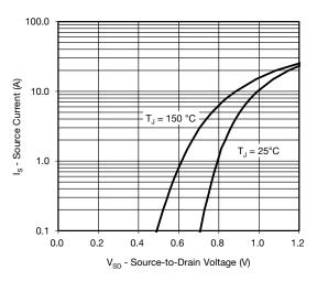
Source-Drain Diode Forward Voltage
