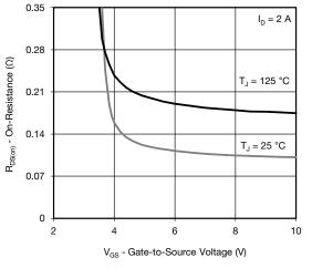
On-Resistance vs. Gate-to-Source Voltage
