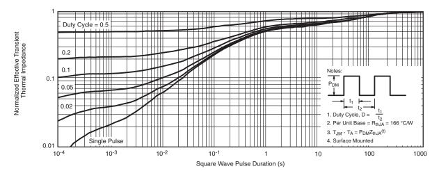
Normalized Thermal Transient Impedance, Junction-to-Ambient
