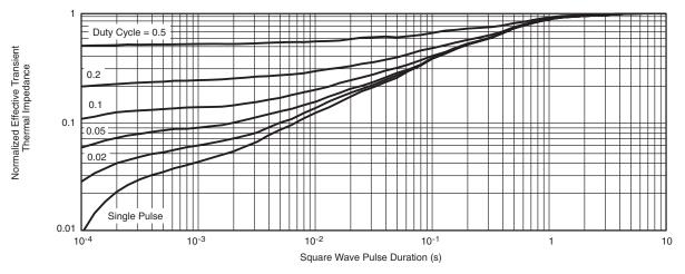
Normalized Thermal Transient Impedance, Junction-to-Foot
