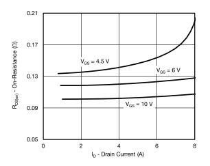
**On-Resistance vs. Drain Current and Gate Voltage**
