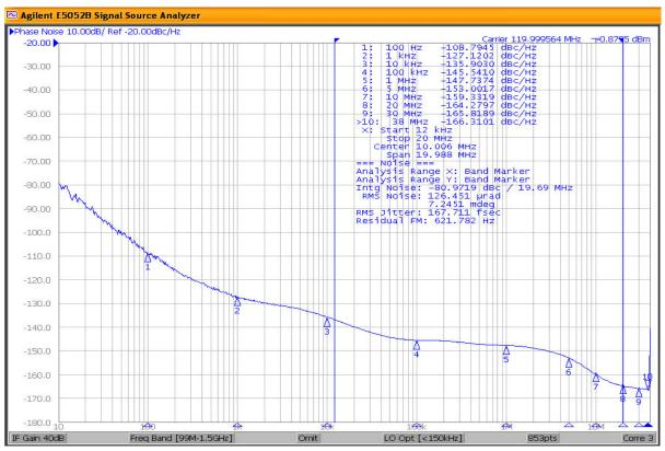
Figure 2. LVDS Output 120MHz 12kHz-20MHz 168fs
